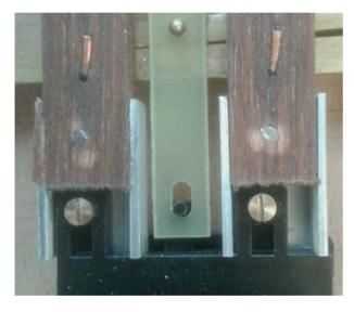
The flick box / motor is offered up to the channels ensuring correct alignment with the tie bar slot and the mounting holes are drilled through the channels and the bolts inserted.
