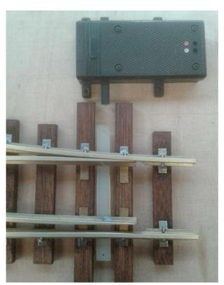
It is obvious that the long sleepers stop the operating arm of the EPL unit from reaching the tie bar.
