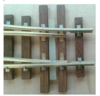
Picture 2, (below left) is a close up of the standard Tie Bar as fitted to ALL stock GRS points.
