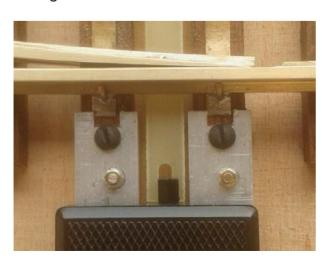
The point is turned over (below left), the nuts are fitted and tightened up and correct operation and free movement is established with a little tweaking as required.
