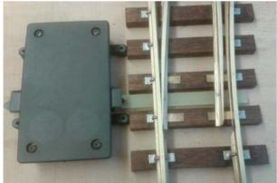
All 3 units require the same Tie bar and it should be stated that all, including the tie bar, can be fitted to either side of the point and facing towards the toe end, or the frog end as required by customer specification. Previously, point motors were attached to the points with a plate, riveted through the sleepers, with the plate underneath and the motor held down with 4 nuts and bolts.
