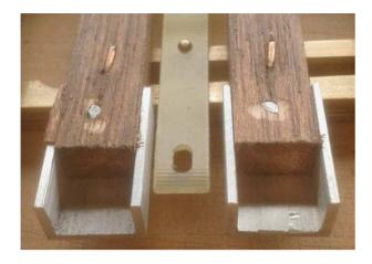
In this picture the channels have been fitted to the sleepers with screws and the excess length of the screws ground off flush.
