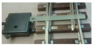
This picture shows the new Tie Bar drilled for fitting to the blades and a SLOT in the end of the Tie Bar where the operating arm of the Flick Box, the EPL unit or the Train-Line motor will locate.
